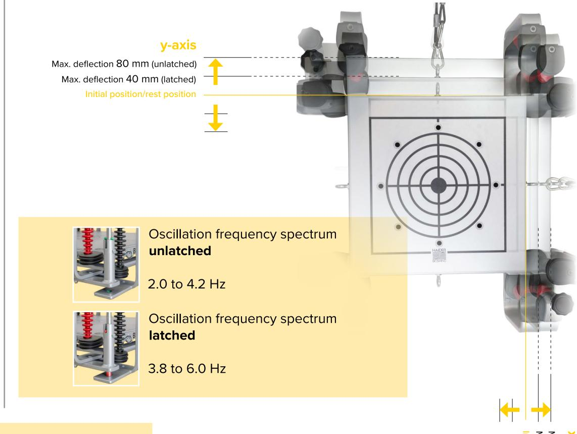
The higher the oscillation amplitude, the more demanding the exercise! Resistance progression in the deflection of the oscillating platform is important for the therapy.
